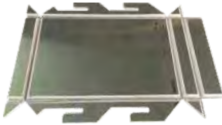
1. Cut and routing the panel according to the standard geometry.
